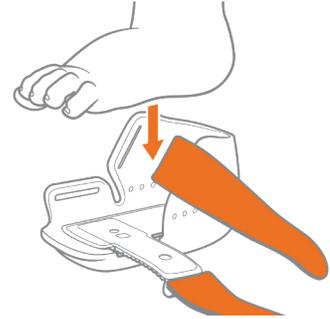
2. Wrap the cloth straps for the boot and the sensor around the foot and feed the straps through the openings in the boot.
